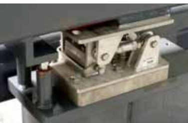
RTN load cells adapted to the application case
