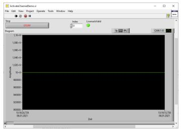
Here we activated a CAN channel that has not been configured correctly before. Because of that, the measurement values are all invalid (delivering 1000000 as value).
