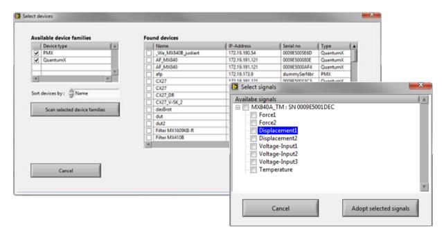
Common device commands, e.g., device scan, channel selection, connect, start or stop measurement are realized by common VIs. So main parts of your application can be reused if you change the data acquisition system.
