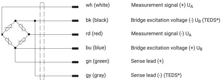
Cable shield, connected to housing
