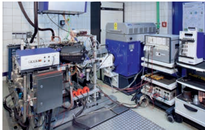
HBM test and measurement equipment in a test bench for hybrid motors at Darmstadt Technical University, Institute for Combustion Engines and Vehicle Drive Systems (Institut für Verbrennungskraftmaschinen und Fahrzeugantriebe (vkm)).
