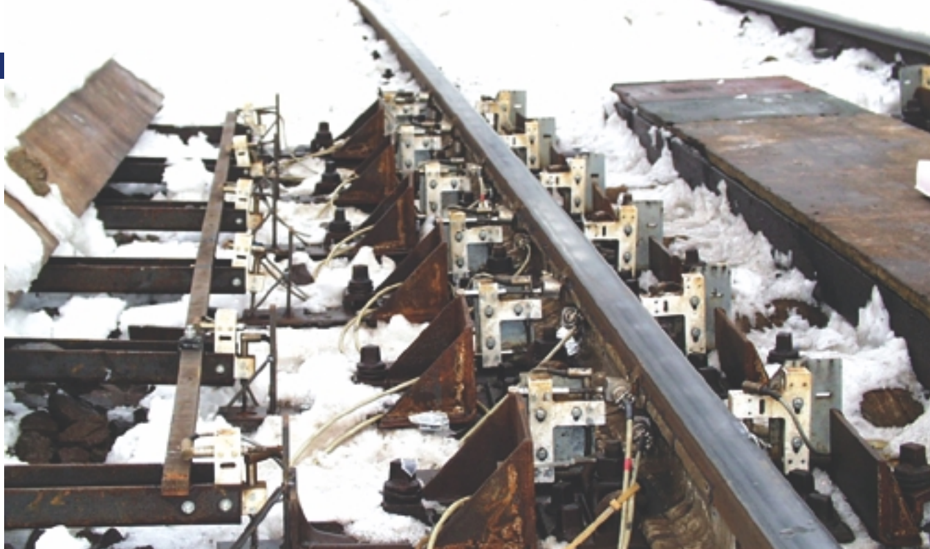
The layout of displacement transducers on a curve
