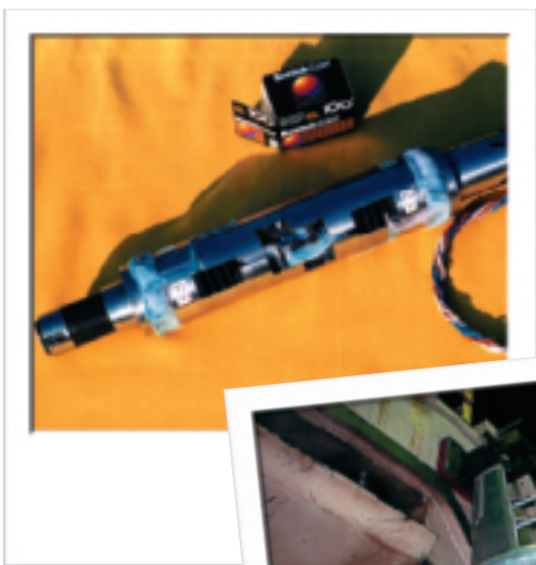
Fig. 2: Internal 6-component wind tunnel balance (color plate)
