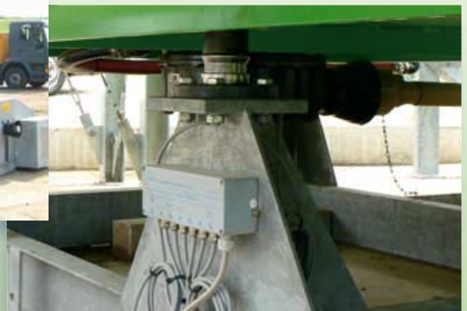
Figs. 2 and 3: RTN load cells with loading foot (above) connected in parallel via junction boxes (below)
