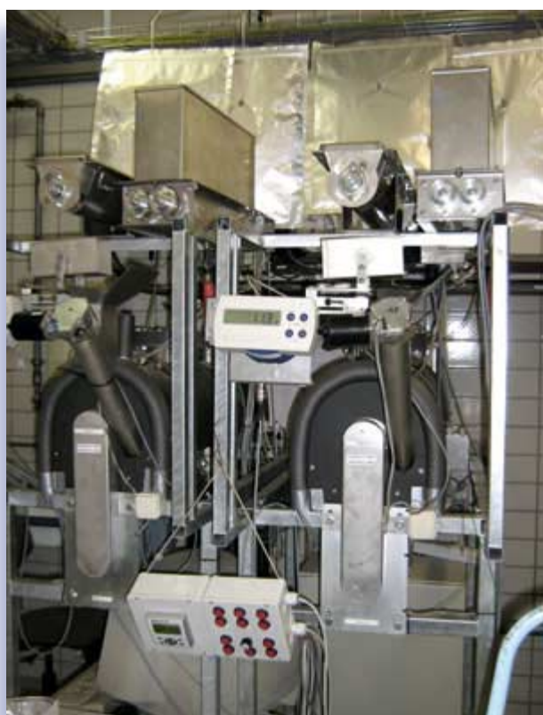
Fig. 1: Automatic fillers for the continuous and automatic operation of lab-based biogas fermenters
