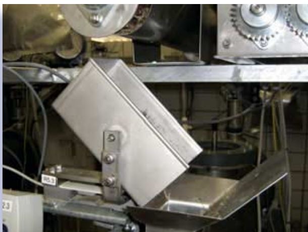
Fig. 2: Scale pan for loading the substrate
