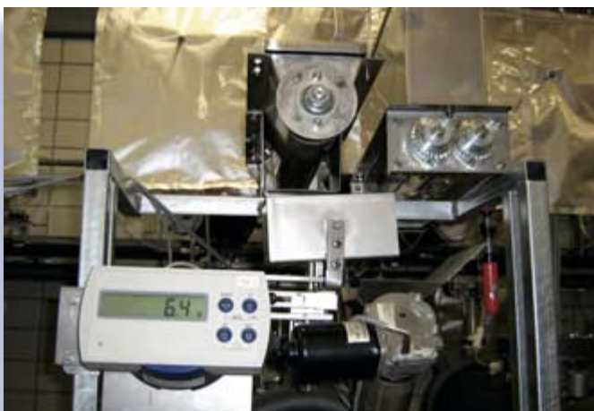
Fig. 3: The HBM WE2107 weighing indicator controls the batching routines
