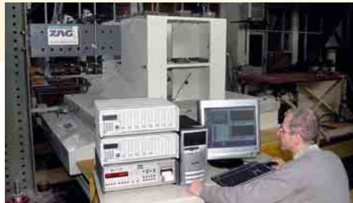
Fig. 2: Function check before the simulated earthquake
