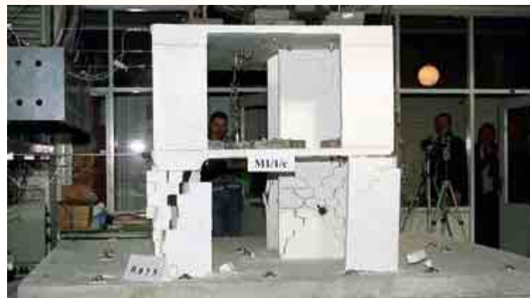
Fig. 3: The last vibration caused by a simulated earthquake
