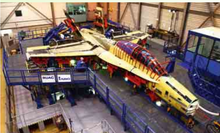
Fig. 1: F/A-18 in RUAG Aerospace test area
