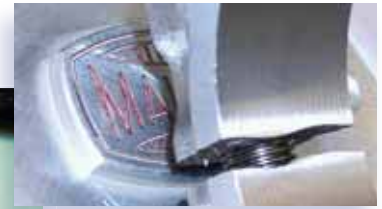
Fracture splitting (cracking) of a conrod at KRAUSE & MAUSER, Germany, the technology leader for this process
