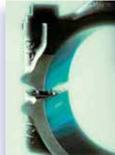
Fracture splitting (cracking) of a conrod at KRAUSE & MAUSER, Germany, the technology leader for this process
