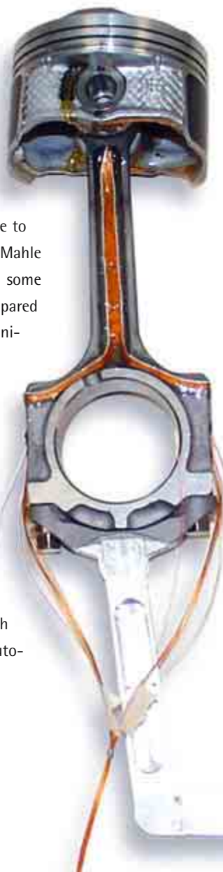
Fig. 1: Piston telemetry system with installed thermistors and signal leads
