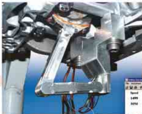
Fig. 3: Fully installed piston telemetry system
