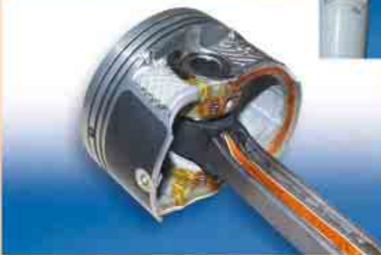
Fig. 2: Eight thermistors are placed under the combus- tion recess of the piston
