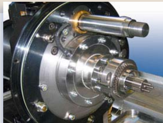
Fig. 2: Transmission test rig with integrated multi-component transducer
