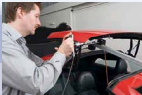
Fig.1-3: Measurement setup on the component test bench for the hardtop
