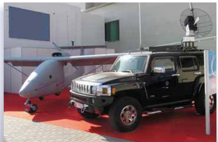
Fig. 6: Unmanned aircraft IAS Archimede UAV with mobile ground station Hummer GCS from International Aviation Supply S.r.l.
