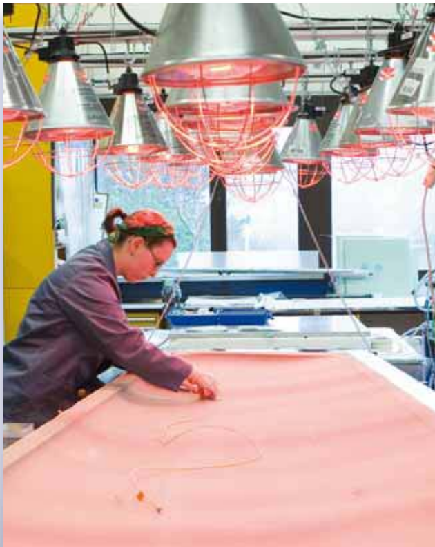
Fig. 2-5: Wing cover made of composite material with embedded sensors. Fraunhofer Institute LBF, Germany
