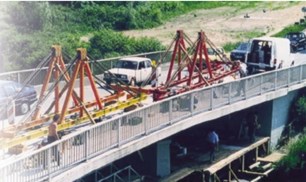
Fig.1: Load testing with the aid of loading frames at Dassow, Germany (1993)
