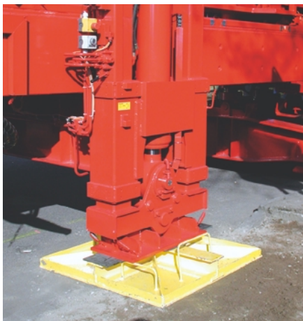
Fig. 9: One of the two front supports with integrated force measurement
