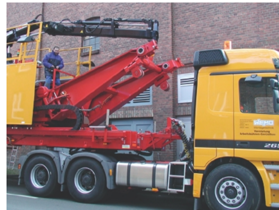
Fig. 4, above: Extending the frame increases the usable length to 18 meters
