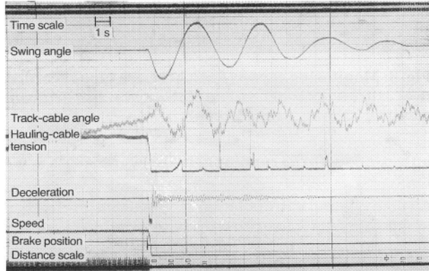
Fig. 10: UV-oscillograph trace shows sudden change in measured values caused by abrupt deceleration
