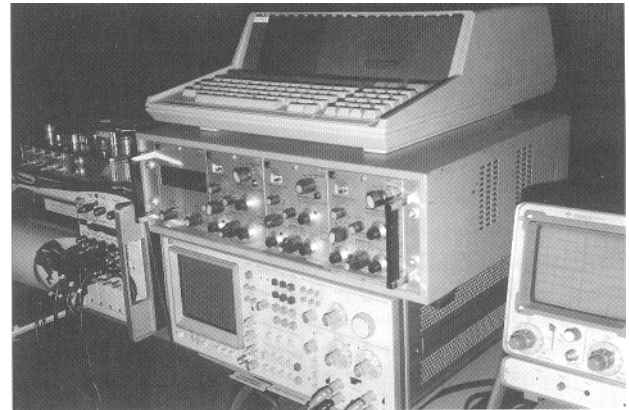
Fig. 3: Instruments used, including the three-channel KWS 382.D4 CF Measuring Amplifier
