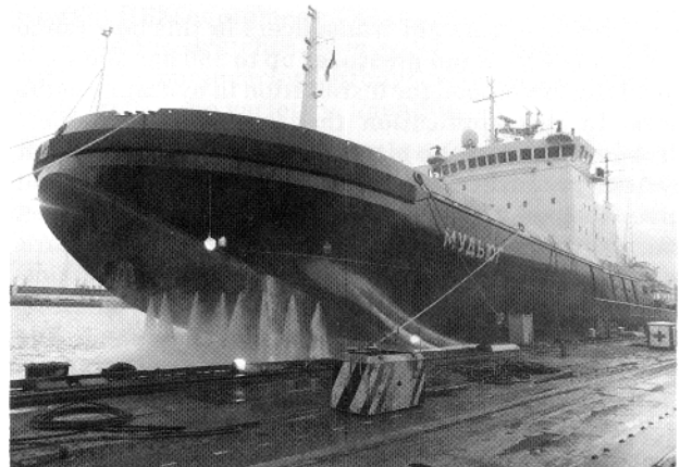
Fig. 3: The ice-breaker "Mudjug" during testing of the compressed-water jets
