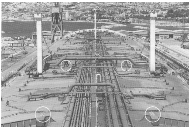
Fig. 1: The top deck of a VLCC showing the points for monitoring deformation
