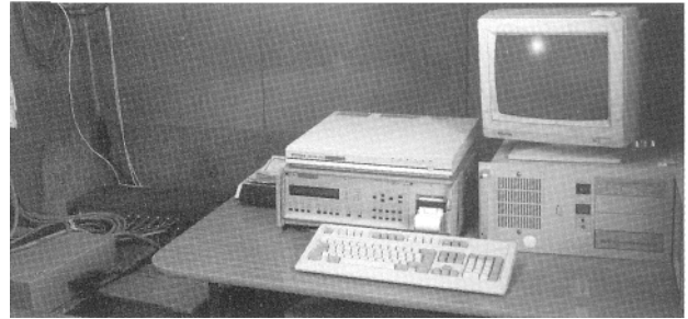
Fig. 12: View in the measurement trailer of the UPM 60 Multipoint Measuring Unit which is connected on-line to a personal computer
