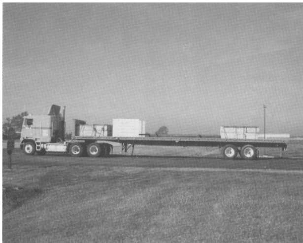
Fig. 8: Test vehicle with a payload capacity of 36 t for the determination of the relative movements in the seal under operational conditions.
