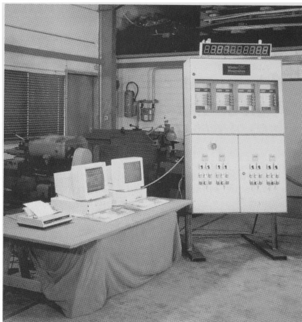
Fig. 9: The system during works trials with the PC for weigher control and evaluation of operational statistics as well as the production of delivery notes and invoices.
