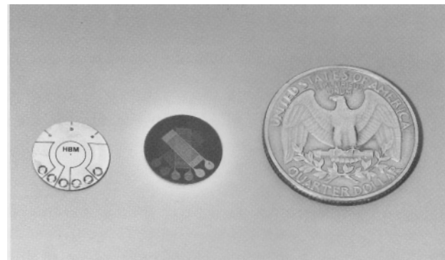
Fig. 3: View of the RY 51 Ring-Core Rosette showing both sides. An impression of its size can be obtained from the quarter-dollar coin.
