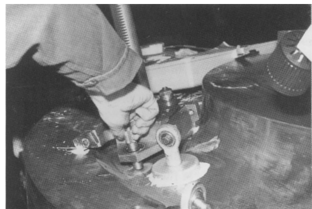
Fig. 4: Central fixing of the support for the milling device above the measuring point.
