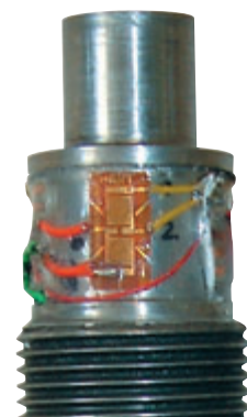
Fig. 7: Front part of the measuring bolt with the T rosette XG11-6/120 SG from HBM, with the pin to which the plate is attached in front
