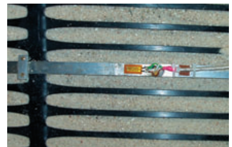
Fig. 9: Exposed spring steel for strain measurement of synthetics, LY11-6/120 SG from HBM
