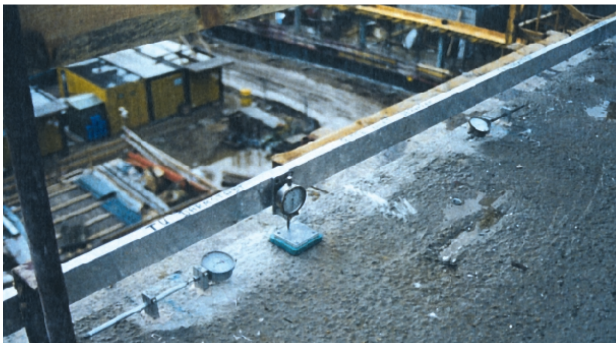
Figure 5: Measuring points for deformation and strain
