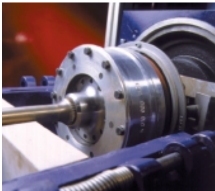
Fig. 5: T10F installed with damping element and flexible connection shaft
