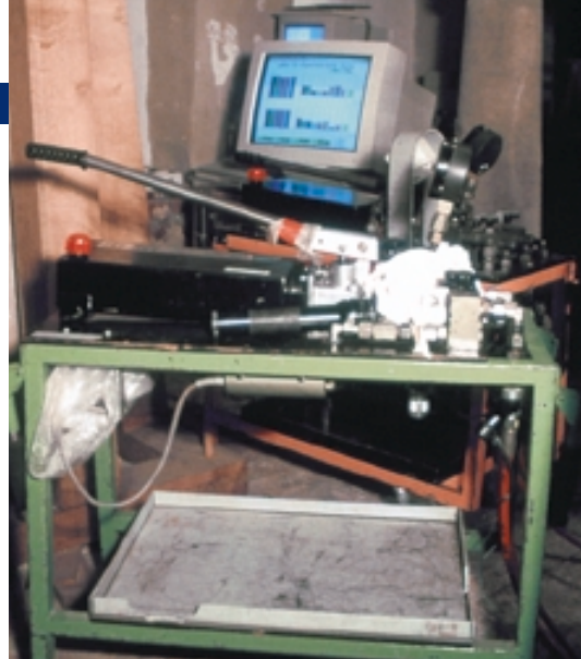
Fig. 10: View of the hand pump for generating pressure; in the background in the field of view of the operator is the monitor displaying measurement data online
