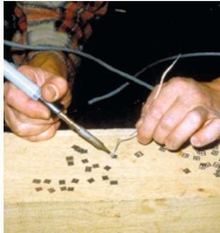
7b: Cleaning and pre-tinning the soldering terminals
