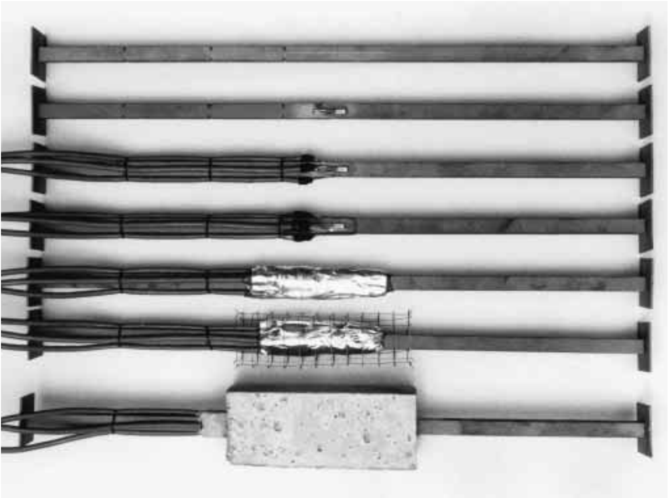
Fig. 10: The measurement transducer used with two S.G.s and a Pt 100 in the individual production phases
