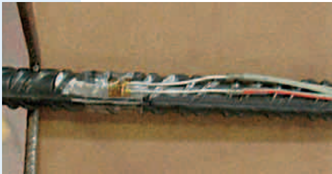
Fig. 7: LY41-3/120 SGs (HBM) for measuring total bar force T
