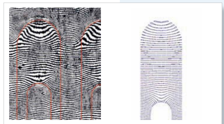
Fig. 10: Isothetic fields for the end loops and links under longitudinal strain from the experiment (Stockmann [2]) and from the FE calculation (Tao [3])
