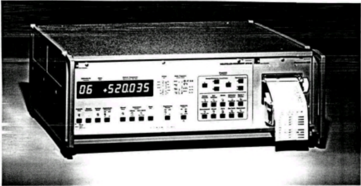
FIGURE 2. Scanning unit equipped with dc and carrier frequency amplifiers to provide highest precision with various transducer types
