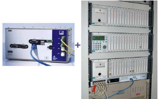
Fig. 13: SI-405 optical interrogator together with MGCplus
