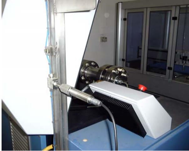
Fig. 6: Use of P3MBP/5000 bar on a high pressure pump
