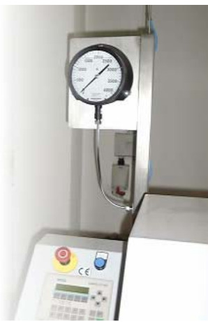
Fig. 4: Conventional pressure gage on a high-pressure pump for a waterjet cutting machine
