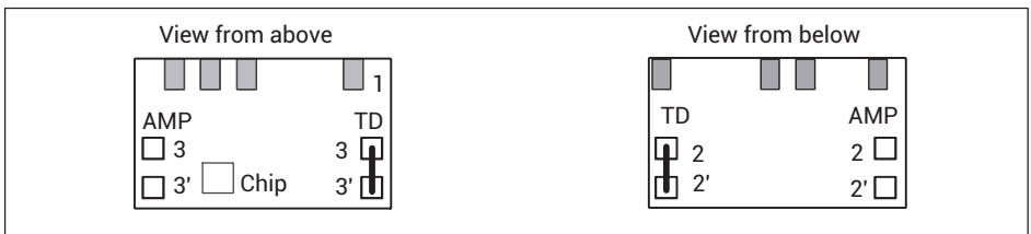
Fig. 2.16 View of TEDS module with pin assignment
