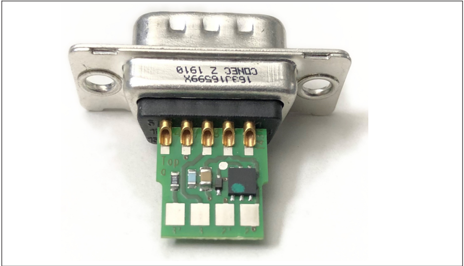
Fig. 2.4 View of the TEDS module in the plug from above before soldering
