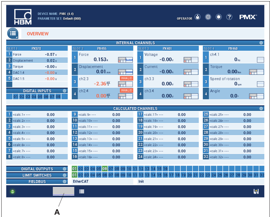
Fig. 11.1 The overview page of the PMX web browser with the device and signal realizations of the connected PMX.
