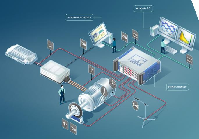
The HBM eDrive Power Analyzers cover the entire measurement chain from high-precision sensors to powerful instruments and intuitive software. And they simultaneously acquire electrical signals like voltage and current, mechanical signals like torque, speed, temperatures or vibration and bus signals like CAN based control commands or test rig parameters. They help engineers to analyze their drive better, faster and more accurately than ever before.
