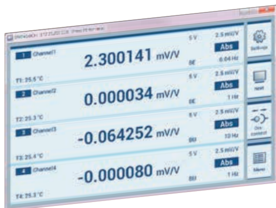
Measurement of up to four temperatures as auxiliary quantities in parallel to the strain gauge signals
