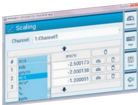
Conversion of the electrical quantity (mV/V) into physical quantities (e.g. kg, N, Nm, Pa) for each channel individually through linearization of 2 ... 11 data points
