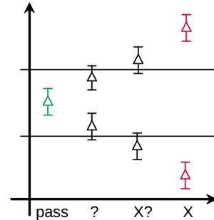
The results on the following pages confirm that the instrument named on page 1 meets the specifications published by the manufacturer and/or agreed by contract that were tested within the scope of the calibration. Measured values with limitations according to DIN EN ISO 14253-1 are marked according to VDI/VDE/DGQ/DKD 2622 as stated below:
