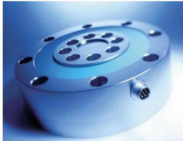
U5 flange-type force transducer. Overhead mounting of the force transducer is possible and, thanks to the flange, it is particularly user-friendly. Nominal (rated) forces up to 500 kN are available. Tensile and compressive forces can be measured.
