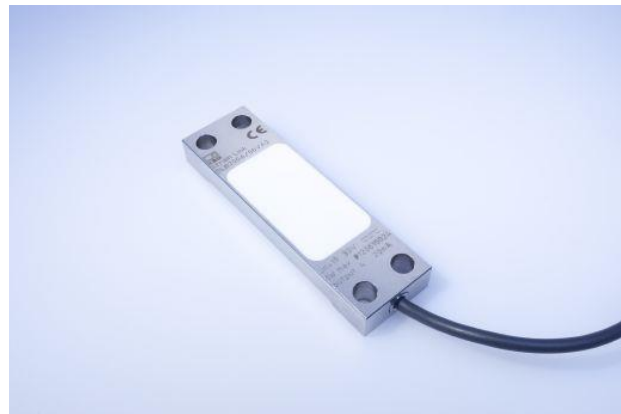
SLB700A/06VA strain transducer. The sensor has been thermally compensated and is ideal for parallel connection due to its high input resistance, sensitivity adjustment and balanced output resistor.
