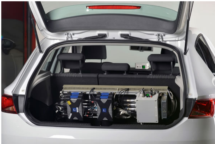
Fig. 1. HBM's QuantumX data acquisition system is designed for structural measurements.
