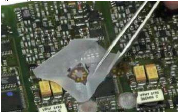
Figure 5: Separation of the Teflon foil after the bonding process
