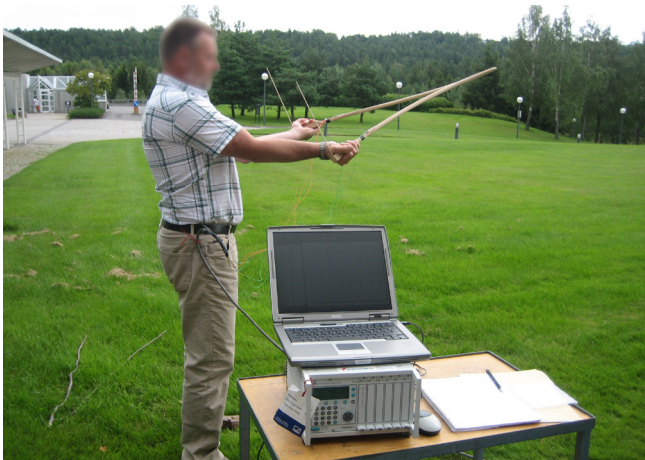
Figure 9: Divining rod instrumented with strain gauges
