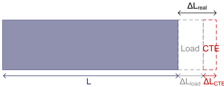
Figure 1 Elongation of a material when subjected to load and temperature changes
