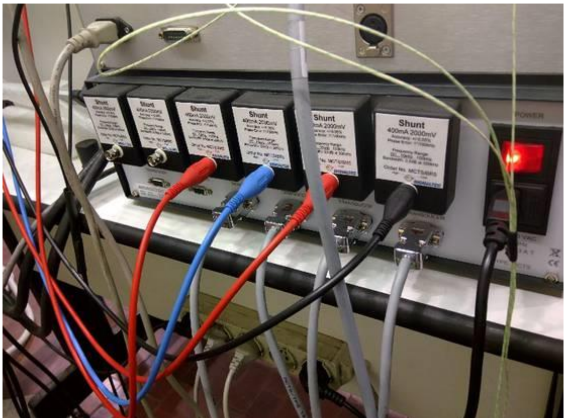
Fig. 3.b: Rear of the current sensors box
