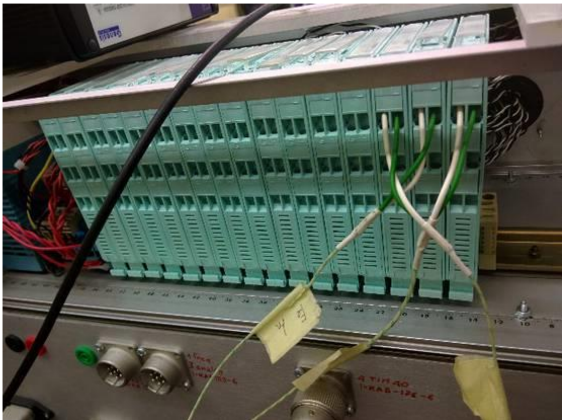
Fig. 4.b: Programmable isolation amplifiers for temperature measurement
