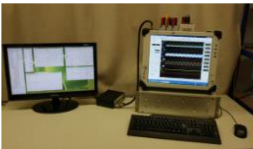
Fig. 6: GEN3i, PC for parameter assignment, current transformer supply and event IO to Txx adapter
