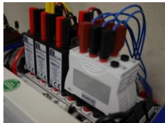
Fig. 7: GEN3i input range with measuring shunts and artificial stars
