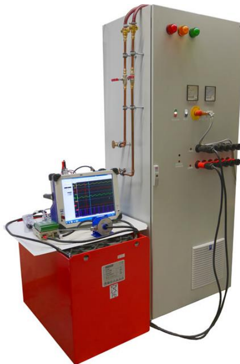
Fig. 6: Proposed High-Performance Test Bench, GEN3i, Pb Traction Battery
