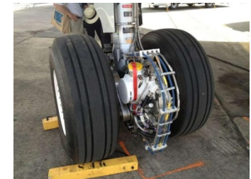
Electrical drive in A320
