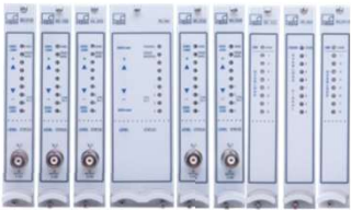
Amplifier boards for 1, 4 or 8 analog channels or special tasks
