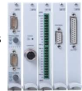
Connection boards for 1, 4 or 8 analog channels or special tasks
