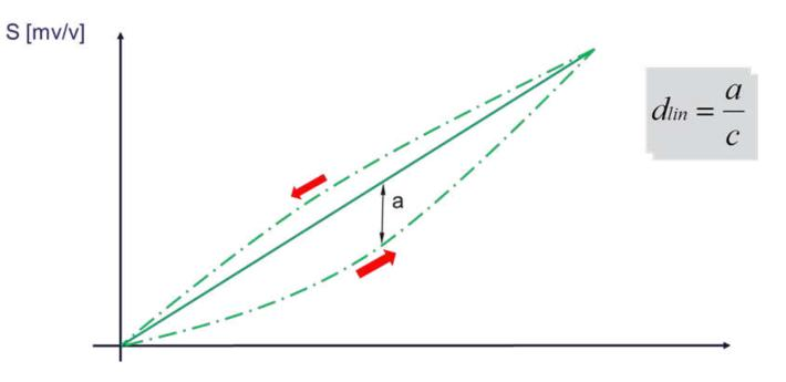
$$\Delta_{d \text{ lin}} = 0,1 \% \text{ of } 5 \text{ kN} = 5 \text{ N}$$
