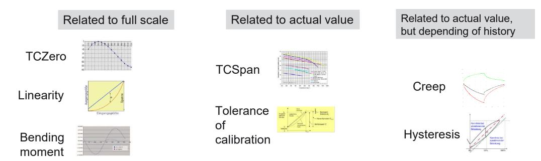
All errors related to full scale have a big impact on measurement of low forces!
